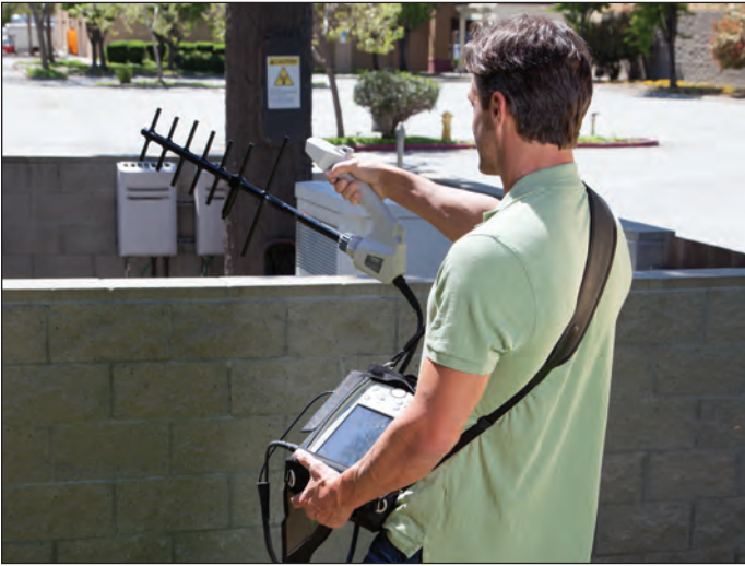
BTS Master MT8220T utilizing MA2700A Handheld InterferenceHunter™.
